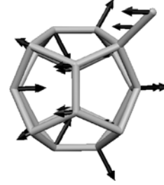
Fig. 4. Displacement pattern of the Tu(3) mode of frequency of 731 cm -1 which gives the strongest peak in the IR spectrum (cf. Fig. 3 and Tab. 1).
